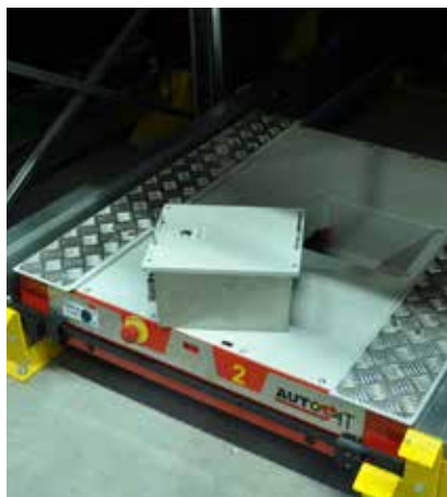
Longlife lithium battery removed for recharging
