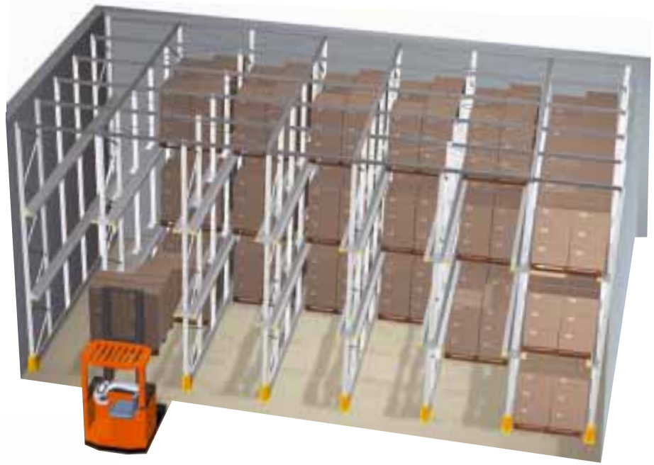
P90 Drive-In racks maximise storage density.
