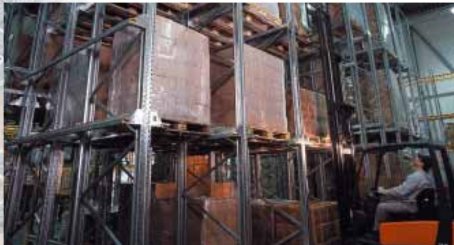
P90 Drive-In racks maximise storage density.
