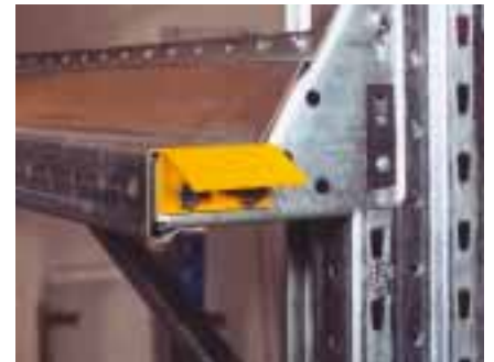
Brightly coloured pallet guides help the driver position the load quickly and accurately.
